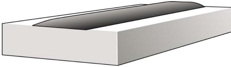
Figure 9 – TherMark™ Laser Marking Material Bonded To The Surface
