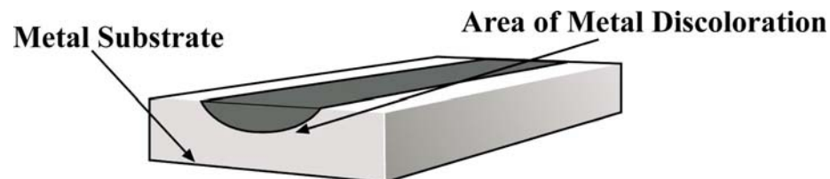
Figure 4 – Marking Applied To Surface Using the Laser Coloration Process
